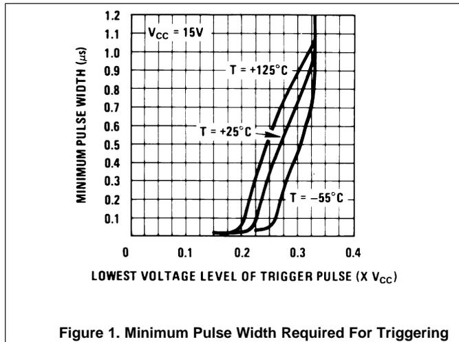
Figure 1. Minimum Pulse Width Required For Triggering
