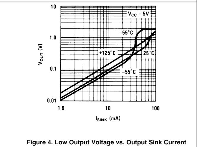
Figure 4. Low Output Voltage vs. Output Sink Current
