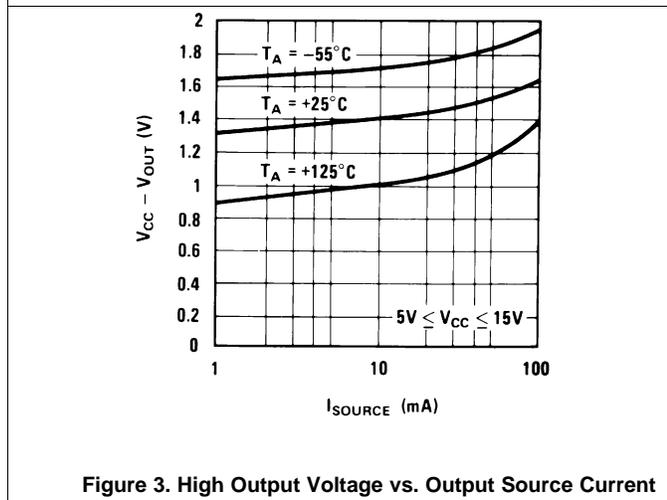
Figure 3. High Output Voltage vs. Output Source Current
