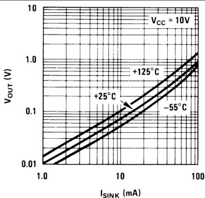
Figure 5. Low Output Voltage vs. Output Sink Current
